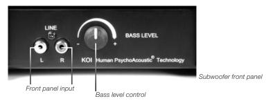
There are three sets of stereo inputs on the Tiger. The **Line** input on the front panel and the **Aux** input on the rear panel of the subwoofer are recommended for use with most consumer audio equipment. The **Audio** input on the rear panel is better suited for pro audio equipment with standard OdBu (.775V) line-level output.
